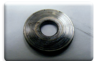
This marking is evidence of contaminated oil
