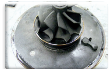
Turbine end oil leakage due to restriction in oil drain
