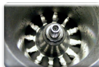
Any object sucked into the compressor will damage it
