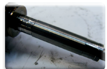
Extreme wear on the turbine shaft
