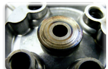
Scored and discoloured surface due to insufficient oil
