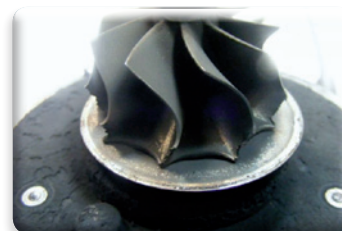
Damaged blades mean the turbo won't provide boost
