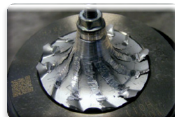
Even small items can completely destroy the blades
