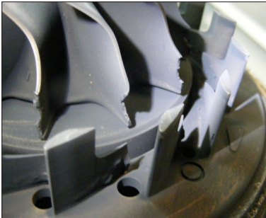
Damage caused by failure of the EGR valve.
