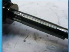
Extreme wear on the turbine shaft caused by oil contamination
