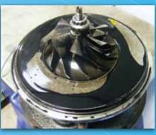
Compressor end oil leakage due to low air pressure
