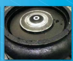
Compressor end oil leakage
